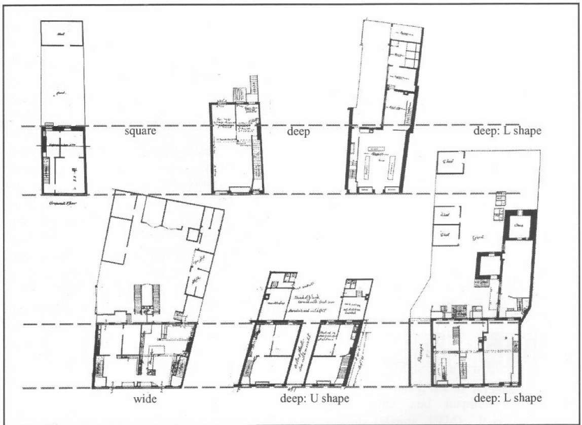
Figure 2. Architectural order: building footprints and ground-floor plans.
