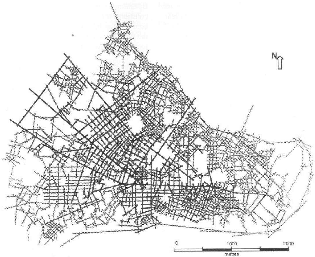
Figure 6. Axial map of the historical peninsula in 1964. The lines are shaded in a continuous scale corresponding to the numerical levels of integration (I). The most integrated spaces are shown in bold black lines, and the most segregated spaces are shown in light dotted lines.
