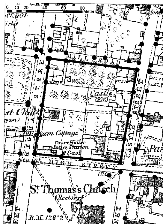
Figure 3. Winchelsea digitized polygon (quarter 8) derived from GPS survey points overlaid on OS First Edition 1:2500.
