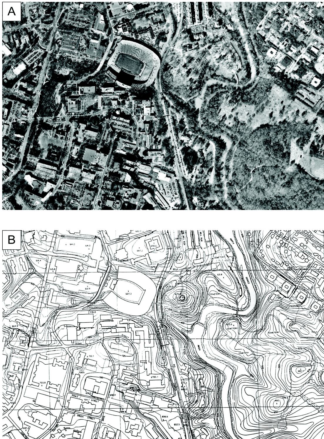
Figure 1. (A) An orthophoto image of the University of Georgia Campus, which can be matched exactly with (B) a large-scale topographic map of the same area
