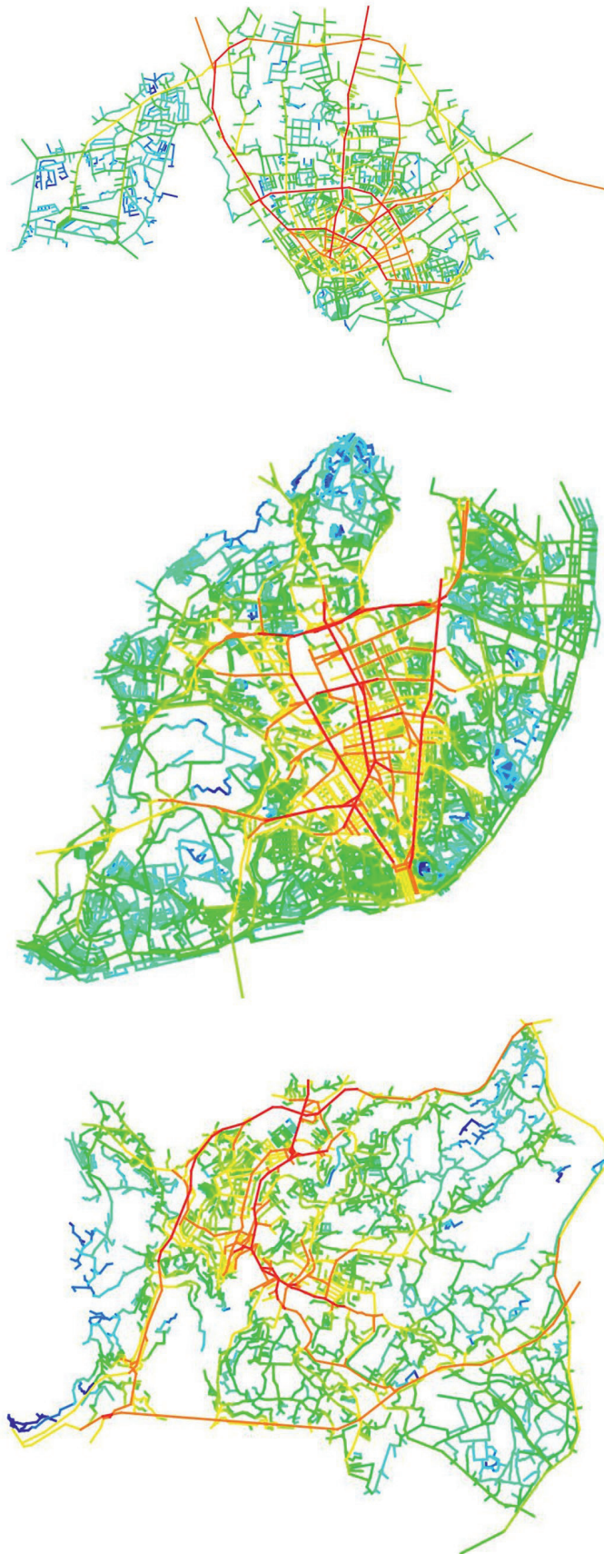
Figure 4. NAIN: the highest values for the background and foreground networks – Faro (top) and Lisbon (middle), and the lowest values for both networks – Vila Real (bottom). In each map, the colour range is from red (highest values) to orange, yellow, green, blue and dark blue (lowest values).
