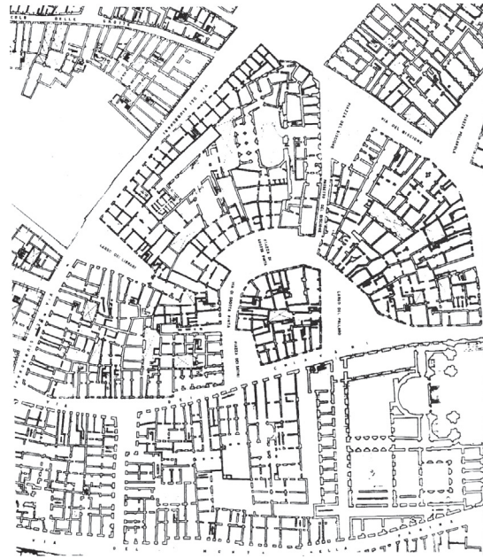
Figure 1. Base building urban fabric formed on the substrata of Pompeii Theatre (source: surveys by the Centro Studi di Storia Urbanistica, 1962).
